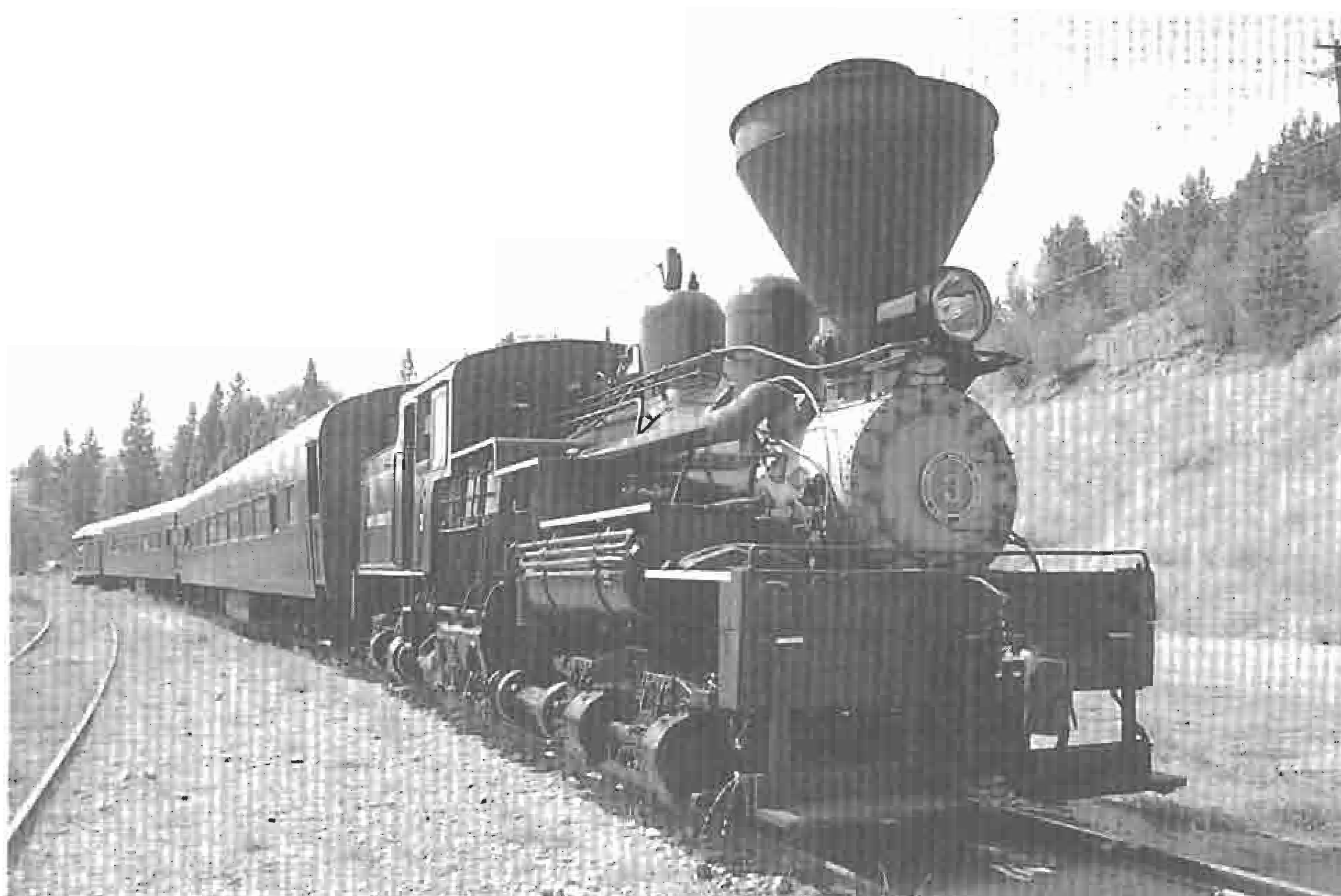
Former Mayo Lumber 50-Ton 2-truck Shay No. 3 pilots a Kettle Valley Railway Heritage Society excursion between Summerland and Faulder, B.C., on August 9, 1999. The two coaches previously operated on BC Rail's "Royal Hudson" excursion between North Vancouver and Squamish, BC. They were built in 1950 as CP 2270 and 2289. The open car was formerly a CP stock car. Photo by Paul Levin.
