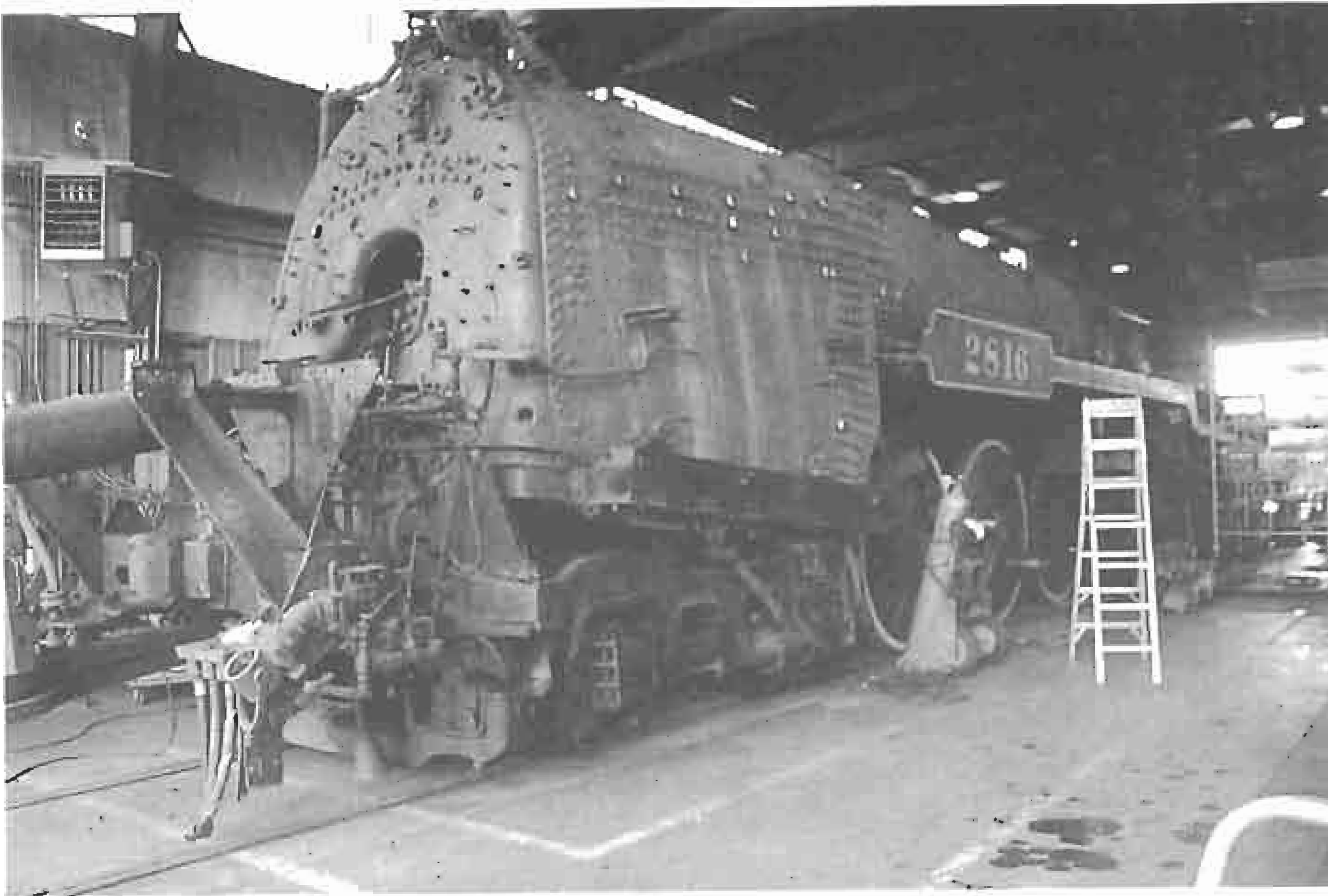
Canadian Pacific standard Hudson 2816, reacquired by CPR in late-1998 after some 35 years as part of the Steamtown USA and later the Steamtown National Historic Site in Scranton, Pennsylvania, undergoes rebuilding in BC Rail's "Steam Shop" in North Vancouver, BC, in August 1999. Photo by Paul Levin.
