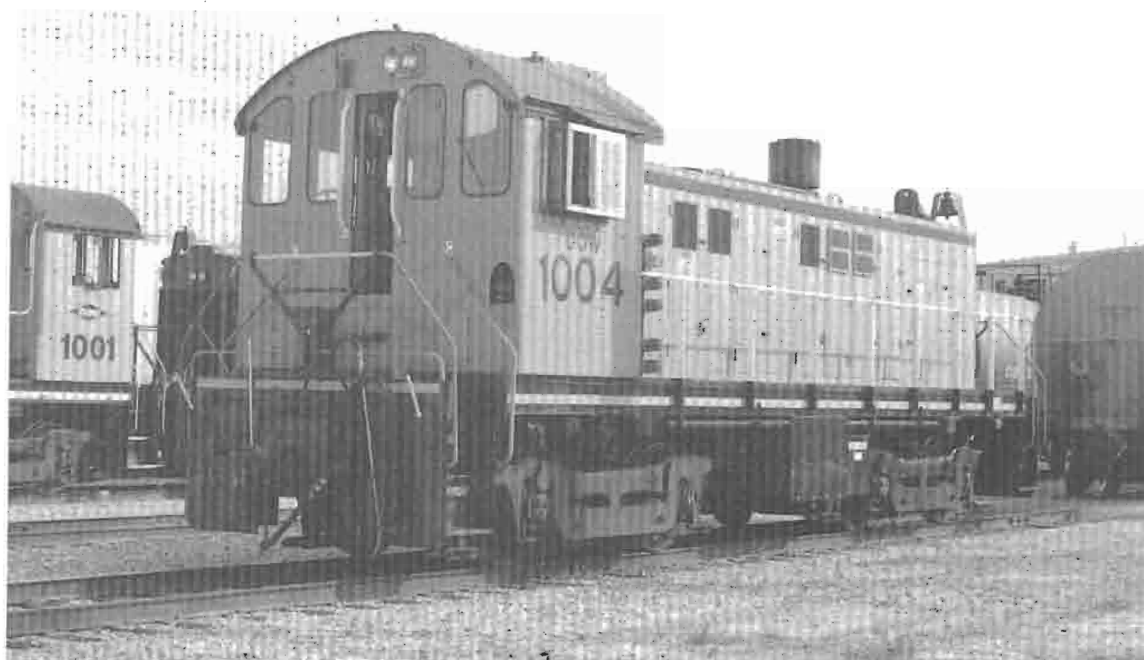
Dow Chemical S-6 1004 is one of seven active switchers at Dow Chemical's facility in Fort Saskatchewan, Alberta. The angles highlights the status lights on the cab sides for remote control. No. 1004 was originally Southern Pacific 1070. Photo on August 7, 1998, by Fred Clark.
