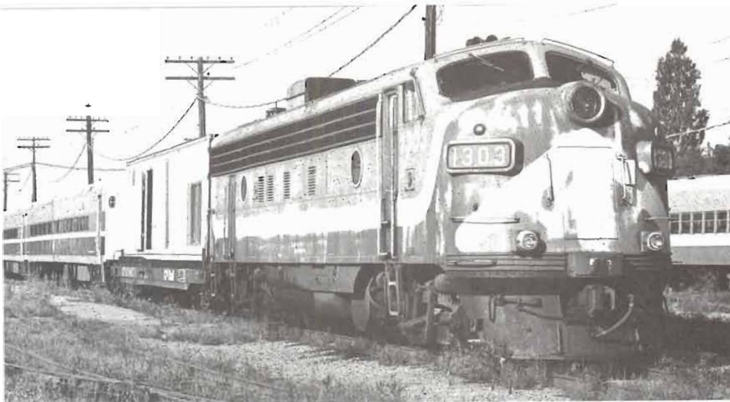
STCUM's somewhat shabby FP7A 1303 (ex-CP 4073) awaits the afternoon commuter rush at Glen Yard on September 6, 1989, two miles west of Windsor Station. Tucked in behind her is a temporary auxiliary power unit on CP container flat 521497. Photo by Ross Harrison.
