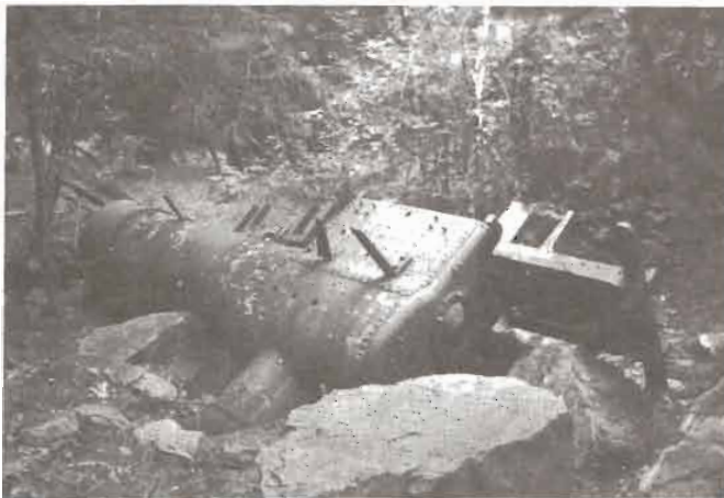
The remains of a 36-inch gauge 2-6-0 used during the construction of the spiral tunnels can be found on Field Hill. Built by Baldwin Locomotive Works in 1885 for the North Western Coal & Navigation, it was abandoned in 1909. Photo by Bruce Blackadder.
