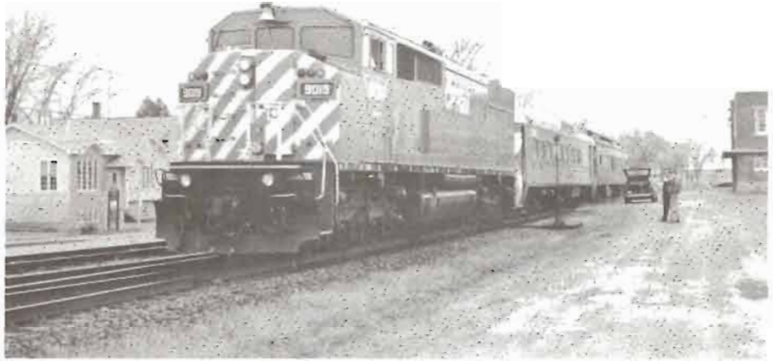
CP Rail Extra 9019 east prepares for departure from Farnham, Quebec, on November 24, 1992. Behind Calgary-based SD40-2F No. 9019 is railway technology exhibit car 91 (converted from RDC-2 9108) and business car "Wentworth". Photo by Raymond Farand.
