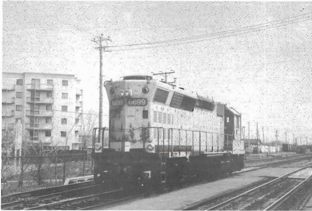
Connecticut DOT GP40-2H 6699 (ex-CSXT GP38 2189) in primer paint, undergoes tests on CN at St-Lambert, Quebec on April 29, 1996. No. 6699 is the last of six former CSXT units being converted for Connecticut DOT at AMF Industries in Montreal. No. 6699 will soon be delivered in "New Haven" livery. Photo by Gerry Gaugl.
