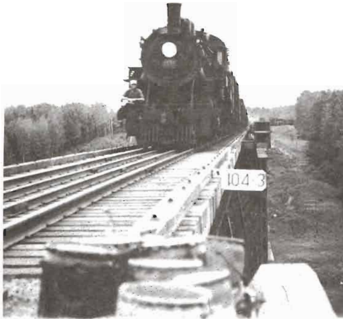
A westbound freight train from Taschereau crosses the Abitibi River bridge, mileage 104.3, in 1943. The headend brakeman is riding the pilot of Consolidation No. 2186 to save time while switching cars en route. The cars will be coupled to the pilot and pushed on to Cochrane Yard, 8 miles away.
