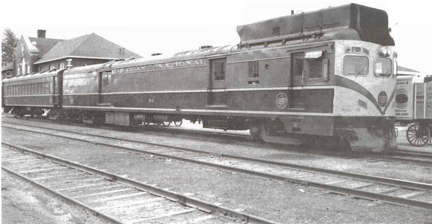
Streamlined Diesel Electric Car D-1 (nee Oil Electric Car 15834) and Trailer C-2 (nee Trailer 15739) on the Cochrane-Kapuskasing run in 1958. The service was replaced by a bus in 1960. The D-1 finished her career as a tower car on the Montreal to Deux-Montagnes electrified commuter line.
